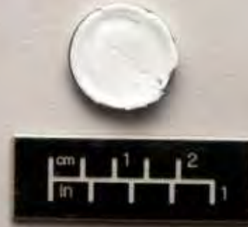
WSTF NO. 14-46305 3M Developmental Material L-14780 Pressure Screen LOX NASA-STD-6001.B Test 13BP Post Purge
