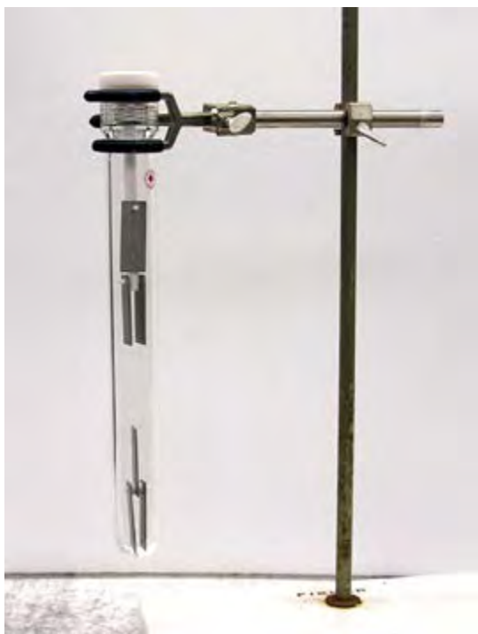
Figure 2. Metal coupons suspended in a high-pressure-rated glass tube.
