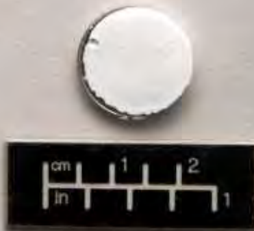
WSTF NO. 14-46305 3M Developmental Material L-14780 Pressure Screen LOX NASA-STD-6001.B Test 13BP Pre Purge
