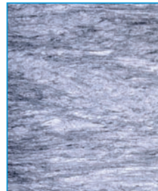
ECAE SFG (<1µm) 100X Dynamically Recrystallized
